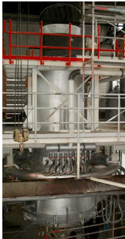
Gas-fired cupola furnace
